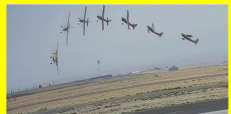
A composite image showing the airplane between 3.7 seconds and 7.3 seconds after takeoff. (FAA photo)
